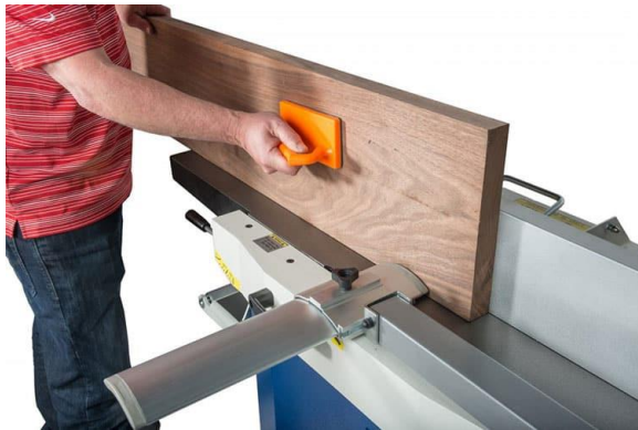
Squaring the edges on a jointer
