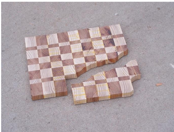
End grain through the planer is not good
