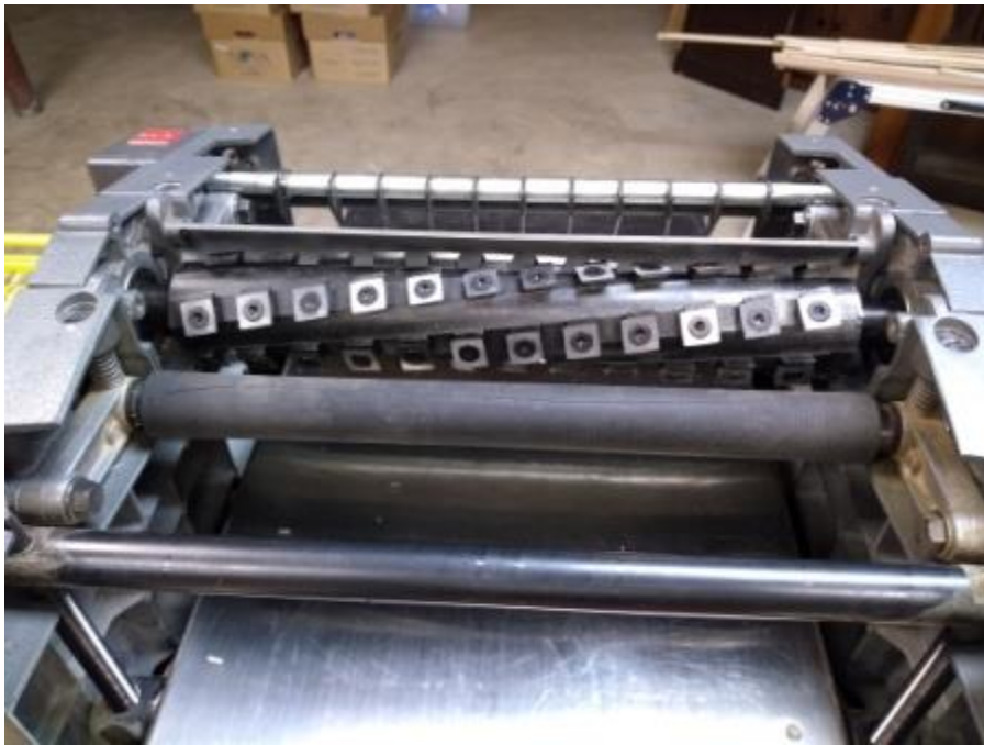
Cutter Head Installed in Planer
